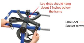
The Leg Ring straps go over the frame, and the black plastic harness clips have a slot that fits over the Shoulder Socket screws. Put your thumb into the round circle and push upward to lock (you will hear it click into place). The round circle will face the ground. The dog's legs go through each ring. To release, put your thumb in the circle and pull downward. Now, you can slowly lower your dog to the ground.
